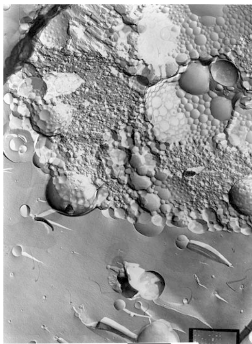
Fig. 5 Freeze–fracture electron micrograph of a complex dispersion encapsulating a 0.05 M saline solution. An oily dispersion of Spherulites (30% w/w) was emulsified in a hydrophilic surfactant aqueous solution (70% w/w). The diameter of the oil globule is about 7 \mu\text{m} . The basic multilayered structure was preserved, but the X-ray diffraction study revealed swelling of the bilayers. The vesicles appeared packed together in the oil globules. Smaller vesicles, probably unilamellar, appeared in the external aqueous phase, probably owing to the presence of some external amphiphiles that were released during the dilution process. The bar represents 1 \mu\text{m}
